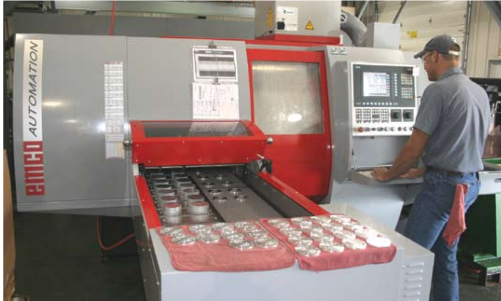
Above: A new EMCO Meyer multi-axis robotic turning center at Pride Mfg.
